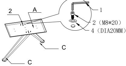
Connect stainless steel base (A) with stainless steel pillar(C) by Bolt(M8X20)
