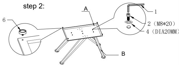
Connect stainless steel base (A) with stainless steel pillar(B) by Bolt(M8X20)
