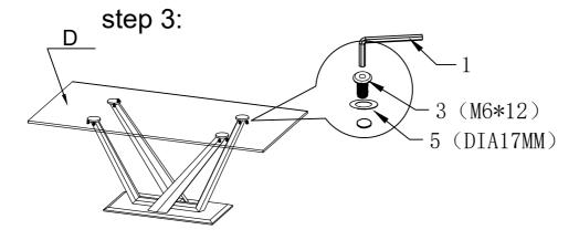
Place the Table top (D) on the Table top frame (C)by Bolt (M6\*12)
