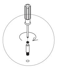
If Cam Lock is too loose, Please adjust Metal Dowel to turn right as drawing.
