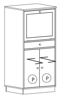
To move door in or out, loosen screw as shown and move door to suit. Re-tighten screw.
