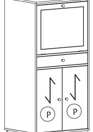
To move door up or down, loosen screws as shown and move door to suit. Re-tighten screws.
