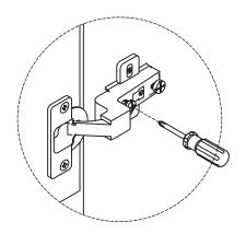
To move doors up or down, loosen screws as shown and move doors to suit. Re-tighten screws.
