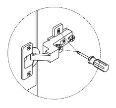
To move doors in or out, loosen screw as shown and move doors to suit. Re-tighten screw.
