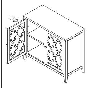
To move doors left or right, loosen screw as shown and move doors to suit. Re-tighten screw.
