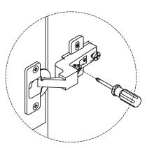
To move doors up or down, loosen screws as shown and move doors to suit. Re-tighten screws.
