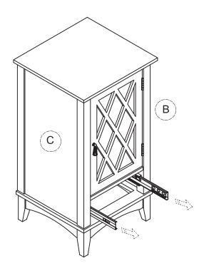
Slide out the side panel drawer glides for proper insertion of the drawers.
