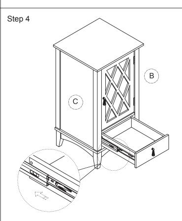
Line up the drawer glides on the drawers on both sides so that they enter evenly into the extended receiving side panel drawer glides as shown then gently push in the drawer until the drawer is secure and slides in and out smoothly.
