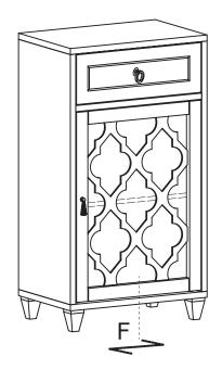
To move door left or right, loosen screw as shown and move door to suit. Re-tighten screw.
