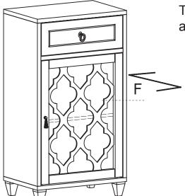
To move door in or out, loosen screw as shown and move door to suit. Re-tighten screw.
