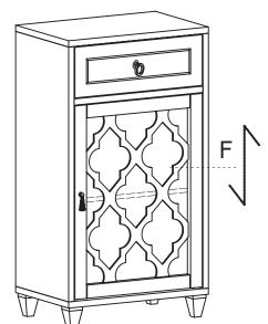
To move door up or down, loosen screws as shown and move door to suit. Re-tighten screws.
