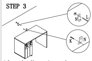
Insert drywall screw into metal bracket and into drywall anchor.
