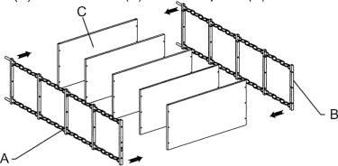
Use the bolt (G) through the right frame (A), left frame (B) and flat washer (I) into nut (H) as shown as drawing and tighten with the wrench (F). Screw the leveler (L) into the bottom of right
