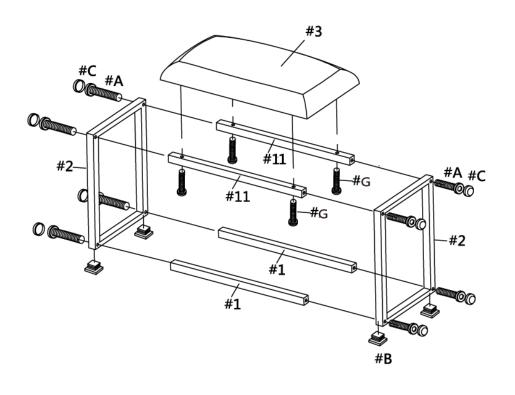
Attach stool side panels (2) to stool top stretchers (11) and stool bottom stretchers (1) together using bolt (A) as shown.
