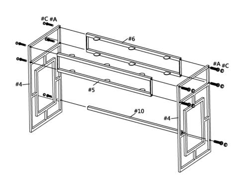
Attach table side panels (4) to table front frame (5), table back frame (6) and table bottom stretcher (10) together using bolt (A) as shown.
