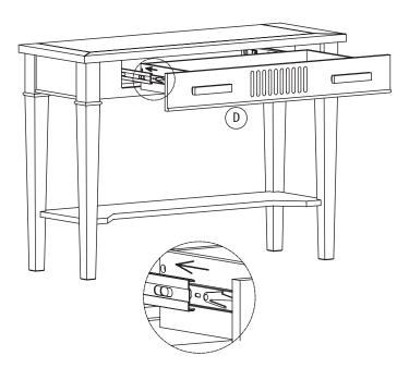
Line up the drawer glides on the drawers on both sides so that they enter evenly into the extended receiving side panel drawer glides as shown then gently push in the drawer until the drawer is secure and slides in and out smoothly.
