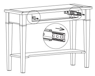
Slide out the side panel drawer glides for proper insertion of the drawers.
