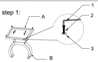
Fit the adjust legs (H) to bottom base, Connect Stainless steel pillar (B) with Stainless steel base (A) by Screw (2) (M8\*50),tighter, one by one
