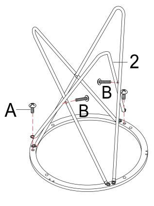
Repeat the step as step 2 that attach last leg (2) to metal frame (1) by using bolts (A) and use bolts (B) to fix all legs together as shown.
