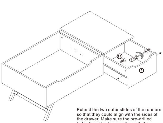
so that they could align with the sides of the drawer. Make sure the pre-drilled holes from the drawer align with the screw holes of the outer slides. Secure two screws from the inside of the drawer using a Phillips screwdriver to tighten them to the outer slides.
