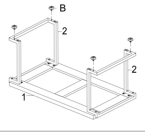
Screw leveler (B) to the bottom of side frame (2) as shown.
