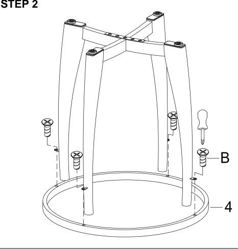
Attach top frame (4) to stretchers by using screw (B) as shown.
