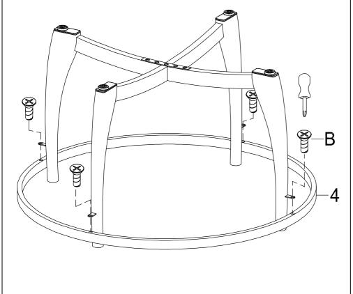
Attach top frame (4) to stretchers by using screw (B) as shown.
