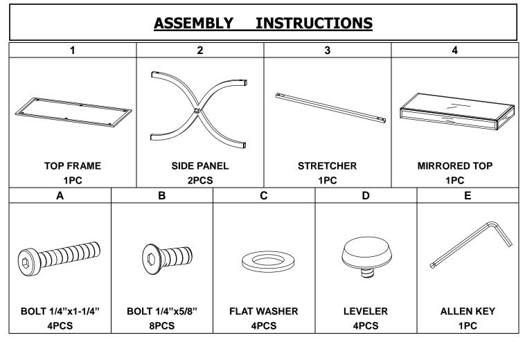
\*\*\* Do not tighten screws & bolts until the entire unit is completely assembled. \*\*\*
