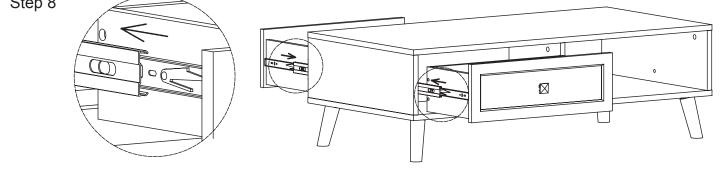
Line up the drawer glides on the drawers on both sides so that they enter evenly into the extended receiving side panel drawer glides as shown then gently push in the drawer until the drawer is secure and slides in and out smoothly.
