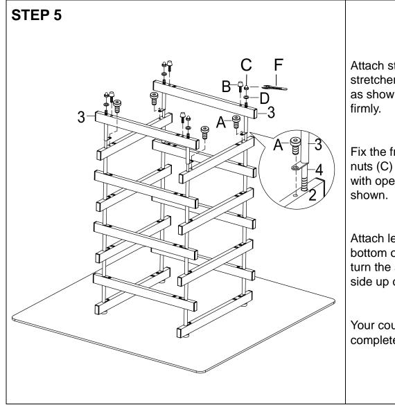
Attach stretchers (3) to stretchers (2) by using bolt (A) as shown then tighten all bolts firmly.
