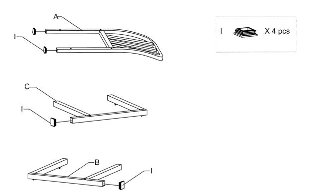
Assemble the chair back (A), left leg (B) and right leg (C) and use the bolt (H) through the chair back (A) into left leg (B) and right leg (C) as shown as drawing and tighten with the wrench (J).
