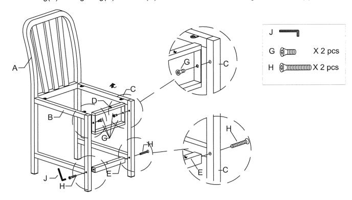
Assemble the seat(F), left leg(B) and right leg(C) with bolt(G) then fastened using allenwrench (J).
