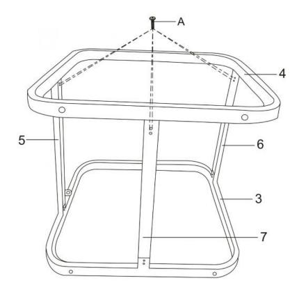
Attach left side panel (4) to the assembled unit by bolt (A) as shown.
