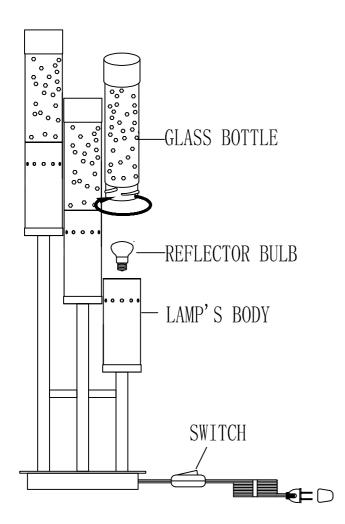
How to replace the light bulb: Switch off and unplug it. wait until the glass tube completely cool down, Remove the glass tube with counterwise, use the suction cap to remove the bulb counterwise from the socket.
