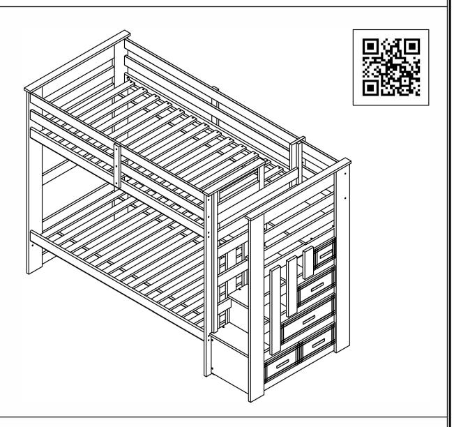
**IMPORTANT**: Do not tighten bolts completely until all bolt are completely lined up and inserted into holes
