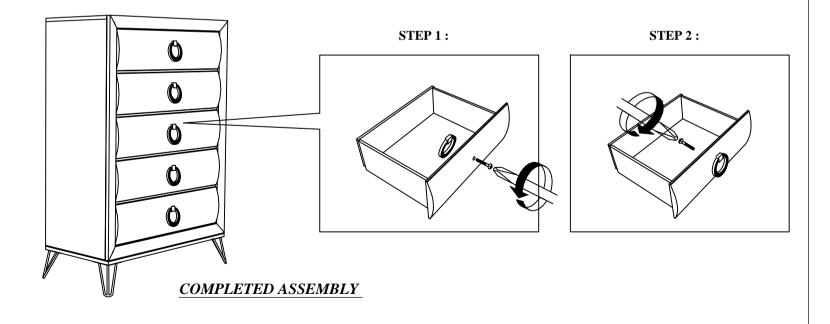
NOTE: MUST TIGHTEN SCREWS PERIODICALLY WITH USE SCREW WILL BECOME LOOSE CHECK TIGHTNESS OF ALL SCREW EVERY 6-8 WEEKS.
