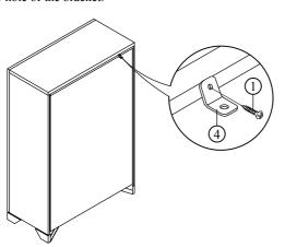
Step 2: Attached the second bracket securely to the wall using the provided longer 50mm screw, through the smaller hole of the bracket. Please attach the second bracket to the wall 2 inches lower than the first bracket that was attached to the back of the chest.
