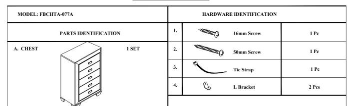
This anti-tipping kit must be attached to a wall using the provided 50mm screws.
