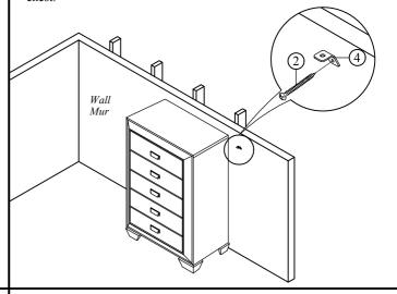
Step 3: Place the chest into position so both mounting brackets are vertically in line. Lace the end of the restraint strap through the bigger hole on each bracket. Bring both ends together and slide the flat end through the locking end and draw it through until all slack is removed. Please make sure that the strap is securely laced and locked.
