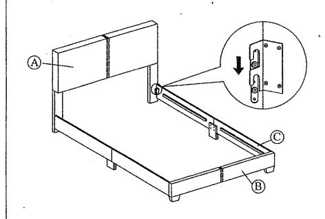
Step 7: Tighten the 4 Corner with Allen Key (6). Install the bed slats to side rail. Tighten the slats with CSK screw. The distance of the slats should be sufficient to obtain desirable bed stability.
