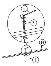
Step 5: Attach side rail (C) to headboard (A) and footboard (B) by gushing the bracket down to fit it.
