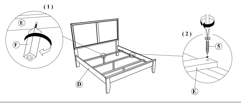
NOTE: MUST TIGHTEN SCREWS PERIODCALLY WITH USE SCREW WILL BECOME LOOSE CHECK TIGHTNESS OF ALL SCREW EVERY 6-8 WEEKS.
