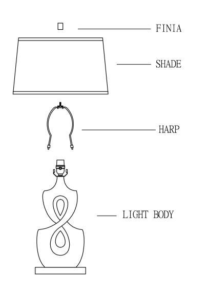
1. SQUEEZE THE OPENING OF THE HARP AND INSERT IT CAREFULLY INTO THE HORNS OF THE LIGHT BODY
